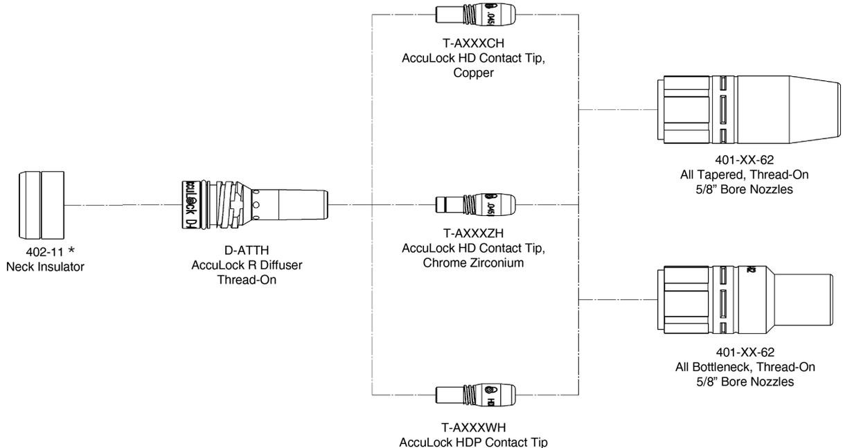
*\*For all Tregaskiss® robotic and automatic air-cooled MIG guns*
